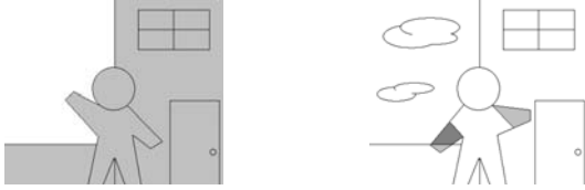
Fig. 1. example of multiple exposure images: (left) high exposure, (right) low exposure
