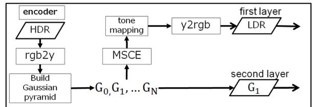
Fig. 1 The block diagram of Jinno's method : (rgb2y)color luminance, (y2rgb)luminance color, (MSCE)Multi-Scale Contrast Enhancement, (TM)tone-mapping, (ITM)inverse tone-mapping
