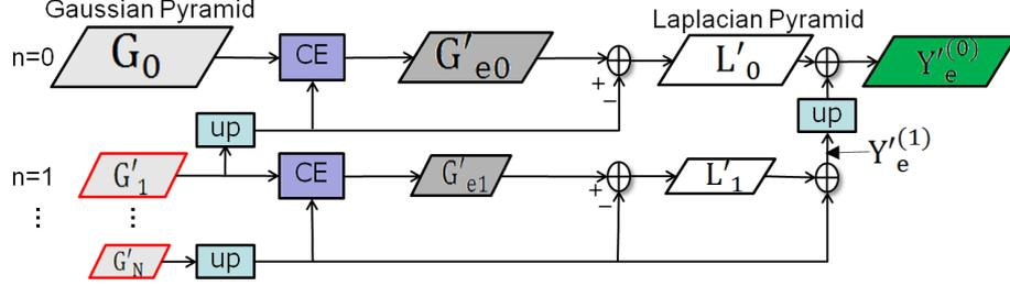
Fig. 2 The block diagram of MSCE
